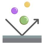
Chemical Inertness/Barrier Properties Insoluble in Organic Solvents, Acids, or Bases, with Very Low Permeability Rates
