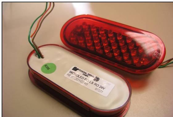
Encapsulation materials can be supplied as either 1 or 2-Part systems using condensation and addition cure chemistries. For a more detailed explanation of these chemistries please refer to the CHT encapsulation application sheet.
