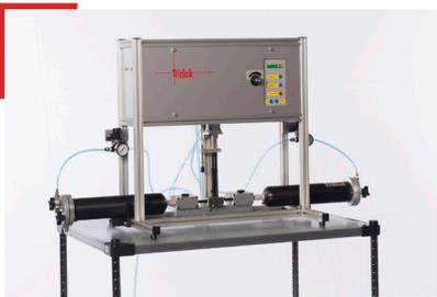
The Tridak® Model 1200 Syringe Filler was designed to fill dual-component syringe cartridges with both materials simultaneously. Ideal for lower volume production or where frequent material change out is required.
