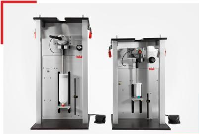
The Tridak® Model 1001 fills syringes, one at a time, quickly and accurately from a material reservoir. It is ideal for low-volume production or as an alternative to filling syringes manually.
