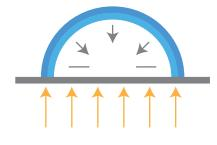
Low Surface Energy (Enables Effective Penetration Under Components)
